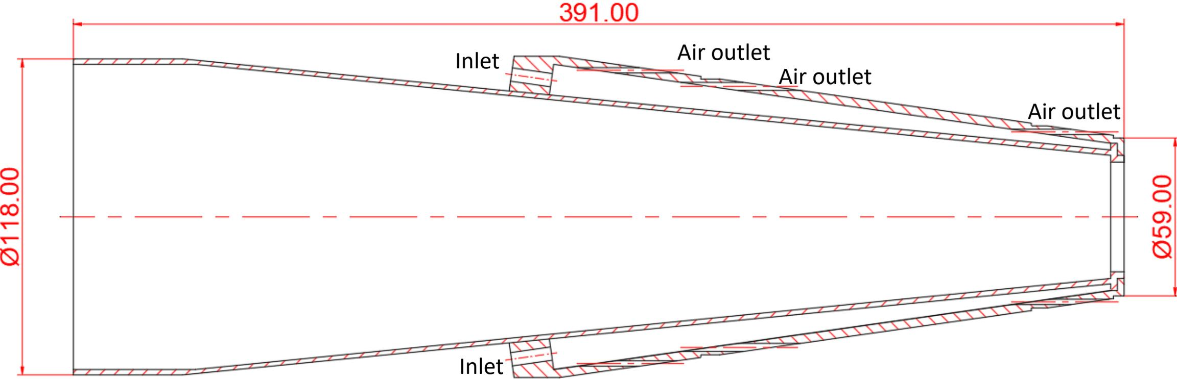
Three "air outlet", each cooling different vertex detectors
