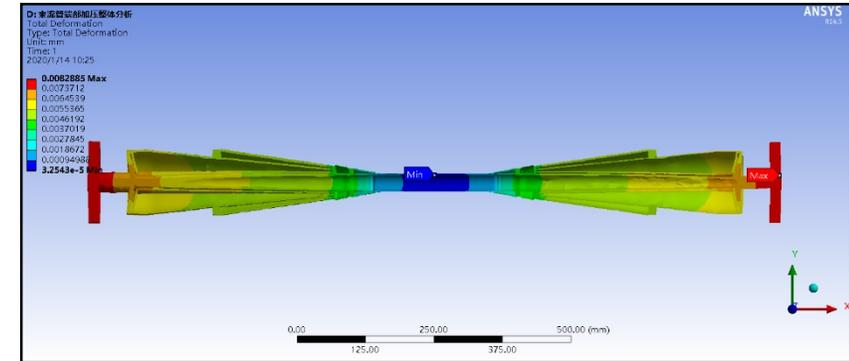
Maximum deformation of end flange: 0.008mm
