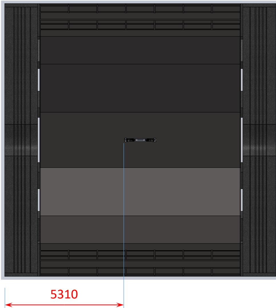
As shown in the figure, the installation of beam pipe in the future is very difficult due to its narrow space, and its axial distance from the center is about 5.3 meter.
