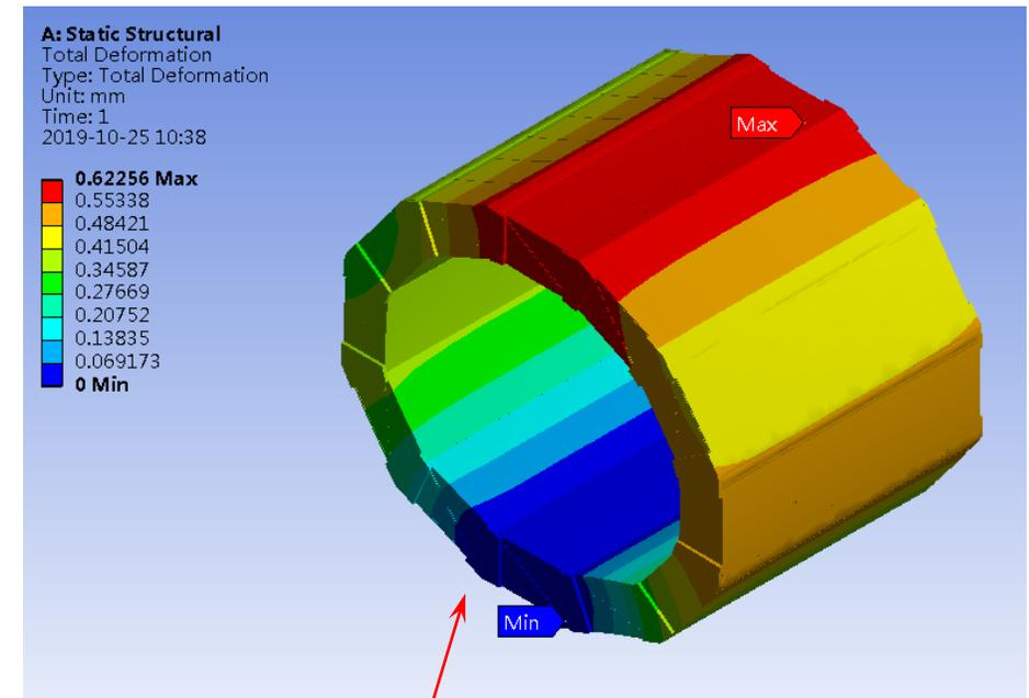
The deformation of its own weight: 0.6mm
