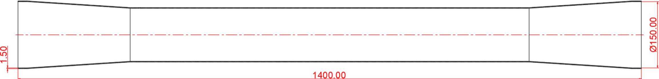
To strengthen the beampipe, at the same time, Carbon fiber cylinder and Gas enlarge channel form the cooling air duct
