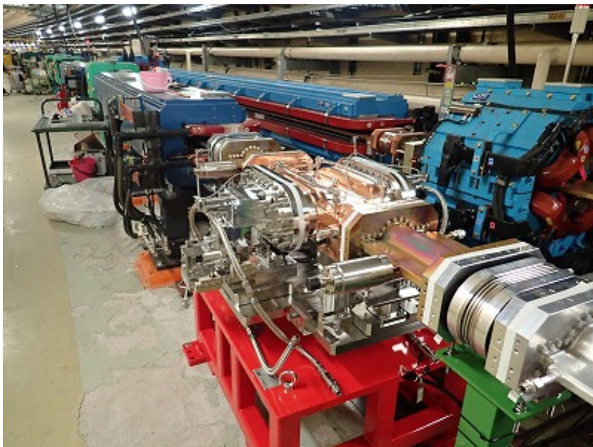
Horizontal type collimator (D02_H1) installed in the LER.
