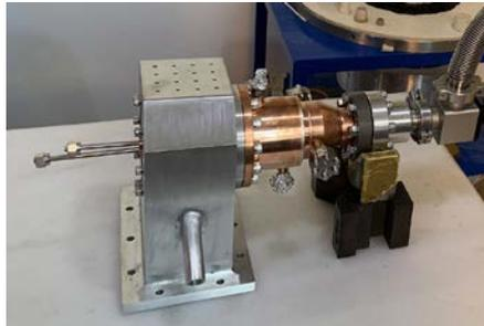
1.3GHz-CW buncher and coupler
