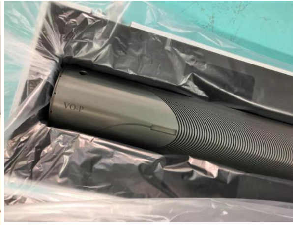
Anodized former and external support tube
