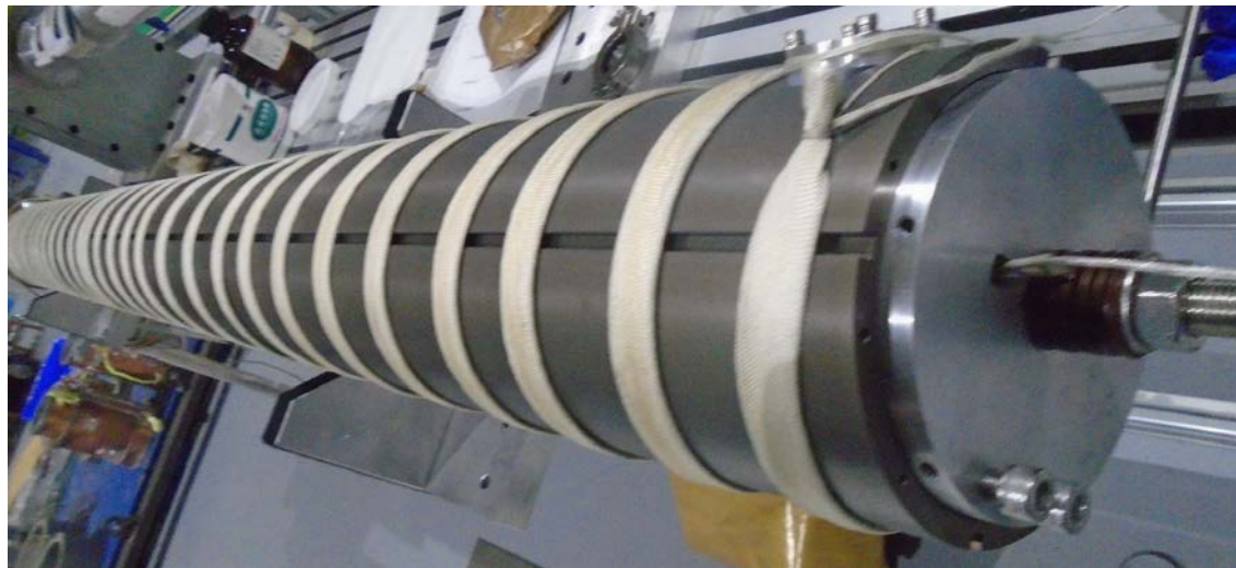
Aperture V coil after VPI
