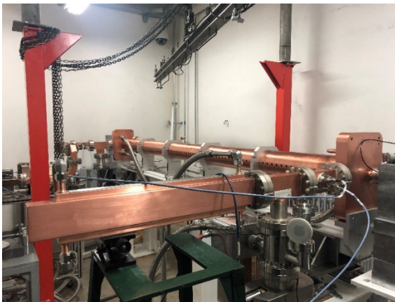
High power test bench
