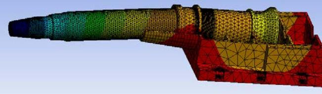
Detailed analyses of the cryostat & support assembly should be done, including the deformation and vibration, considering gravity, temperature, magnetic field force.
