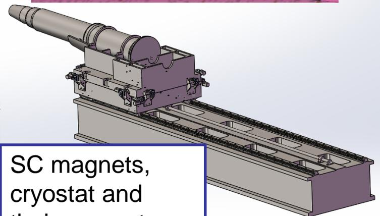
SC magnets, cryostat and their support
