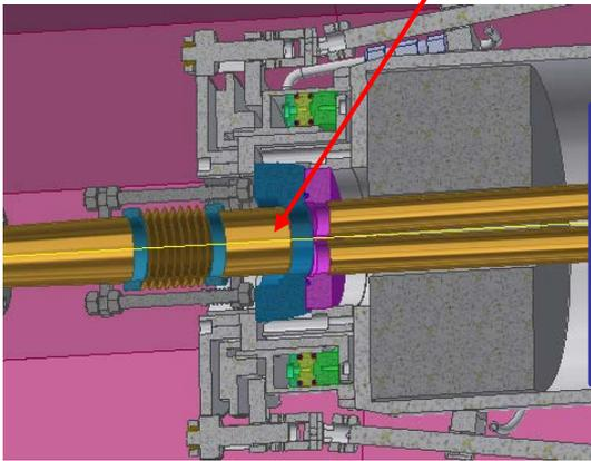
Connection interface of detector and accelerator
