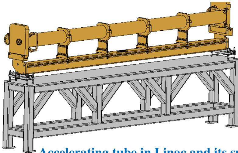
Accelerating tube in Linac and its support:
