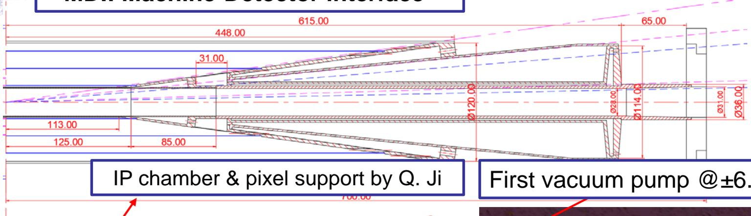
IP chamber & pixel support by Q. Ji
