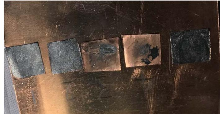
Laminated material with copper and graphene film
