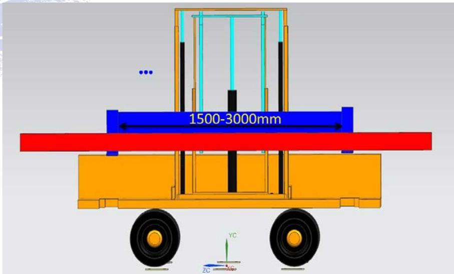
Flexible load support for “long” devices and “short” devices
