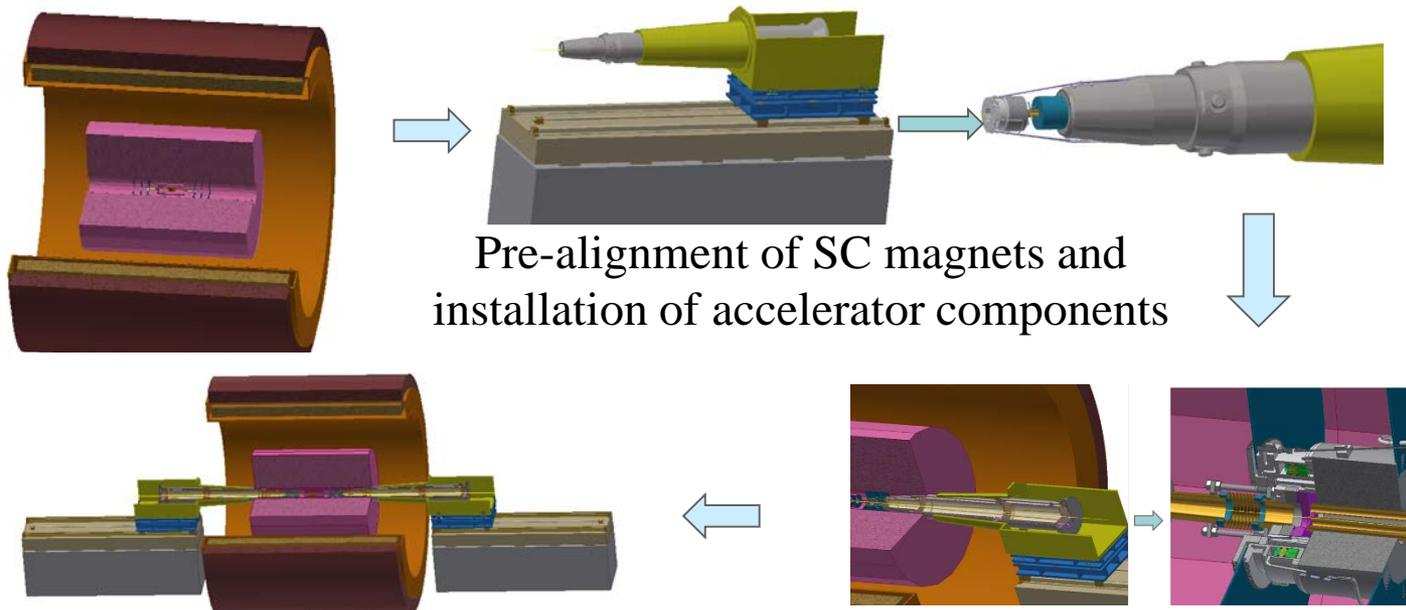
Pre-alignment of SC magnets and installation of accelerator components
