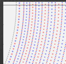
14 co-axial super-layers, 8 layers each (112 total) with alternating sign stereo angles ranging from 50 to 250 mrad, in 24 equal azimuthal ( $15^\circ$ ) sectors
