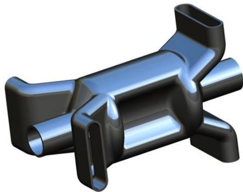
JLab waveguide damped RFD concept
