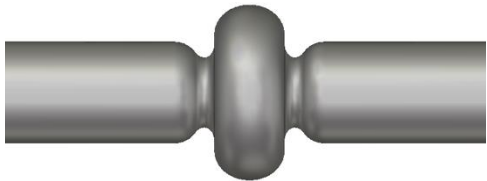
3) enlarged beam pipes
