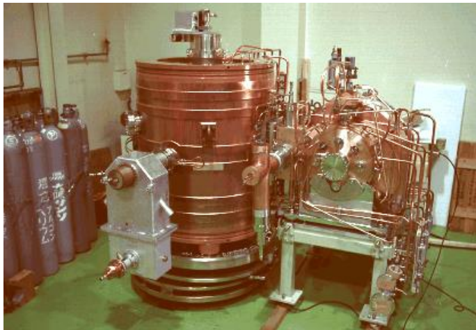
KEK ARES cavity, 508 MHz, 500 kV, 1.75 M \Omega
