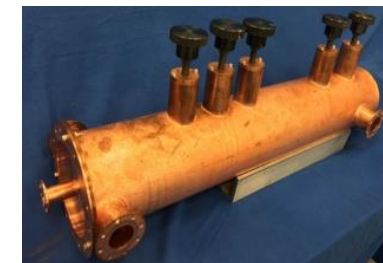
Harmonic Fast kicker for cooling ring
