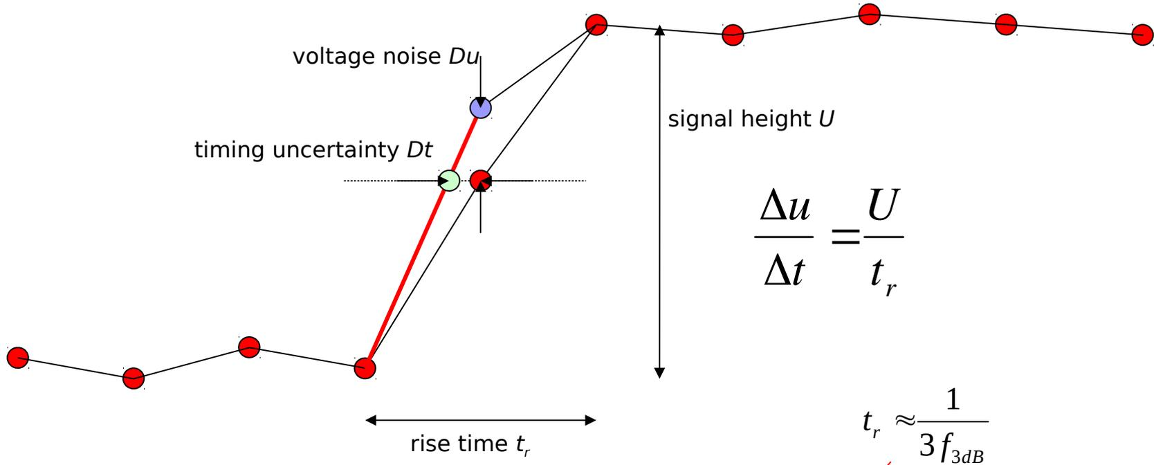
$$\Delta t = \frac{\Delta u}{U} \cdot t_r = \frac{\Delta u}{U\sqrt{n}} \cdot t_r = \frac{\Delta u}{U} \cdot \frac{t_r}{\sqrt{t_r \cdot f_s}} = \frac{\Delta u}{U} \cdot \frac{\sqrt{t_r}}{\sqrt{f_s}} = \frac{\Delta u}{U} \cdot \frac{1}{\sqrt{3f_s \cdot f_{3dB}}}$$
