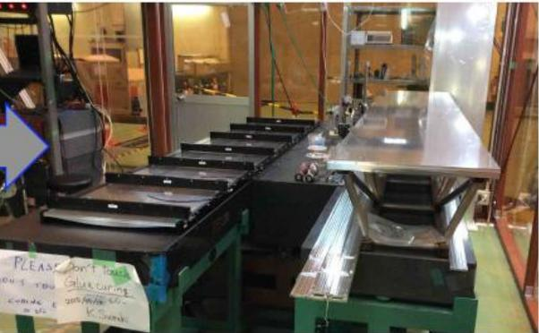
QBB: strong back flattening, button & enclosure gluing.
