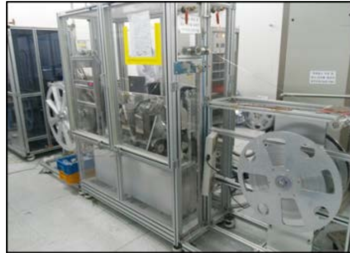
[ Continuous Ic measurement system with Bending-Double bending rollers ]
