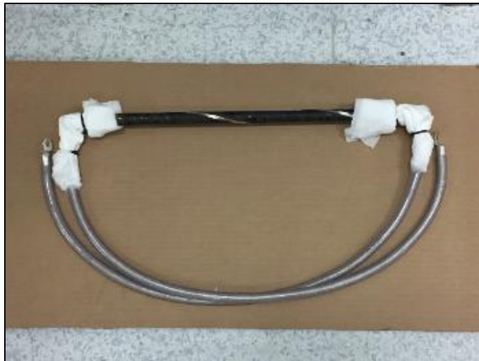
[ Sample based Stranding-Thermal cycle test ]
