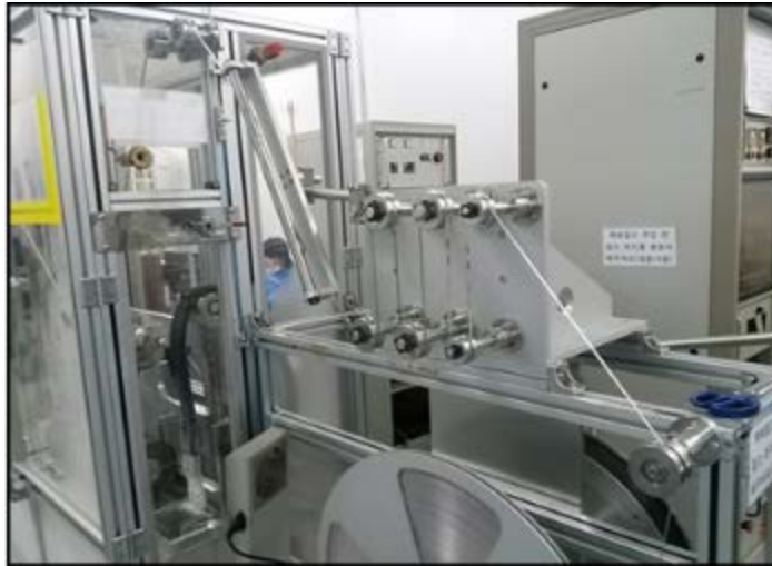
[ Continuous Ic measurement system with Bending-Double bending rollers ]
