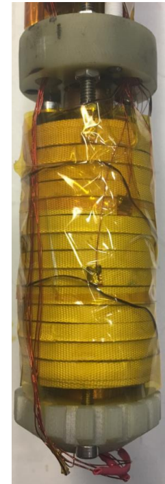
LBC3 HTS insert in 31T resistive magnet reached 45.46T
