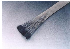
Nb-Ti Rutherford cable with high-precision
