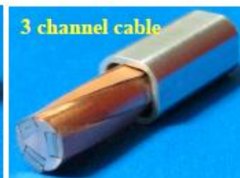
20 YBCO tapes in each helical groove
