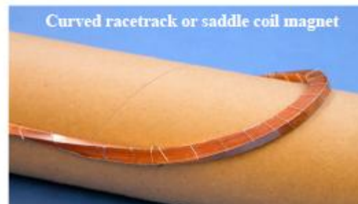
A curved saddle winding of 50 YBCO tapes on a 50 mm diameter tube.
