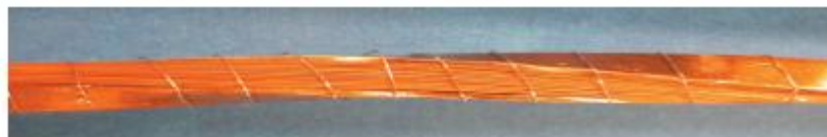
32 YBCO tape Twisted Stacked-Tape Cable (TSTC) with 200 mm twist pitch
