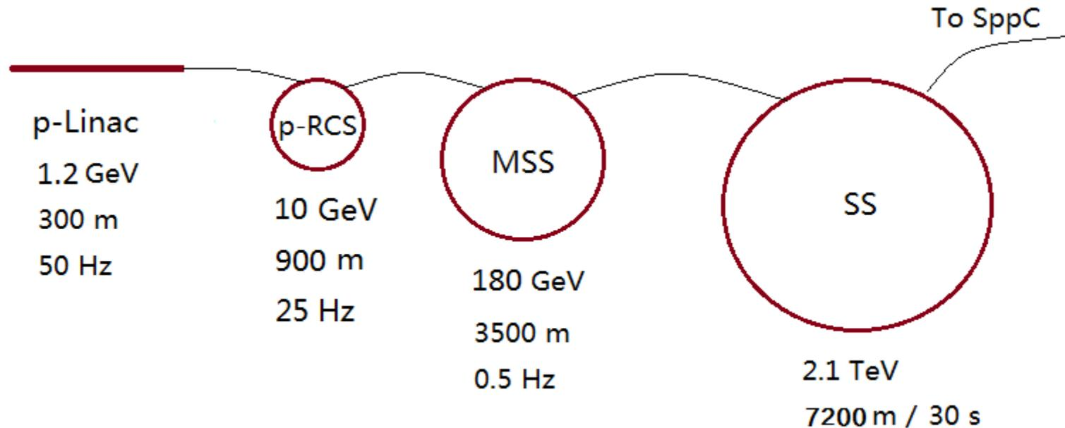
p-Linac: proton superconducting linac
