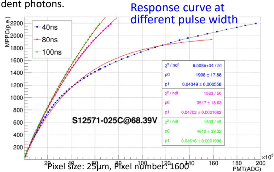
The output linearity of the SiPM are improved with the increase the incident light width.
