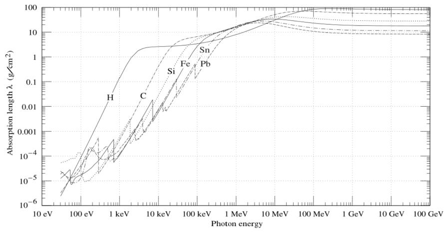
The photon mass attenuation length for various elemental absorbers as a function of photon energy. High energy photons in synchrotron radiation are difficult to shield. Lead is a good material, because it is cheap and has a high density.
