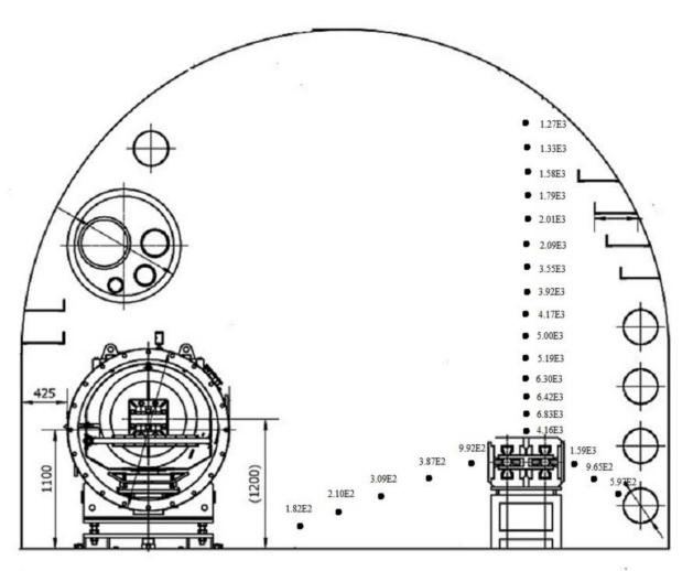
Dose distribution in Gy/Ah at 120 GeV in a dipole section with shielding Radiation dose of the other sections are lower than dipole section.
