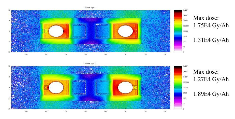
The dose distribution around the dipole coils with lead shielding in different beam directions.
