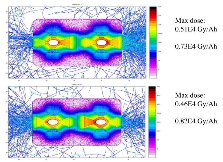
By adding shielding, the radiation dose around quadrupole is significantly reduced.
