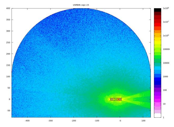
Dose distribution in Gy/Ah at 120 GeV in a dipole section without shielding. The radiation dose around specific equipment such as control electronics, control and instrumentation cable which came closer to the beam line has been estimated.
