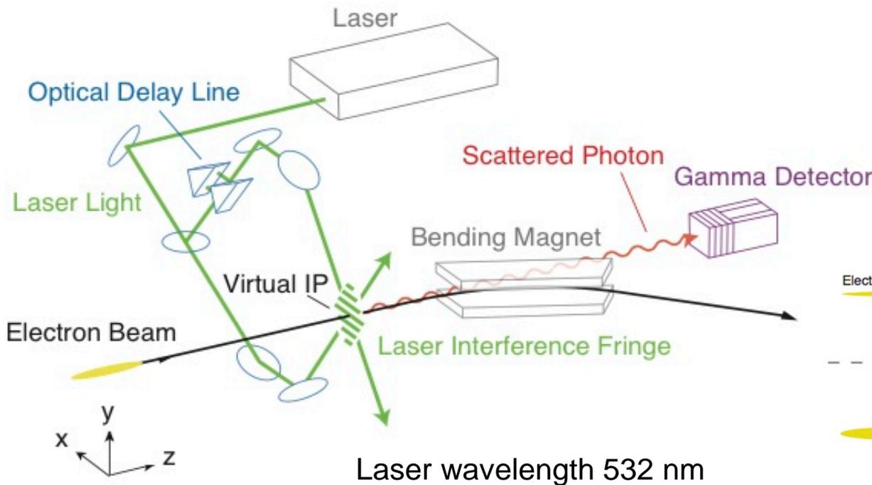
*Modulation of Compton scattered photon rate from beam interaction with laser interference fringe pattern*
