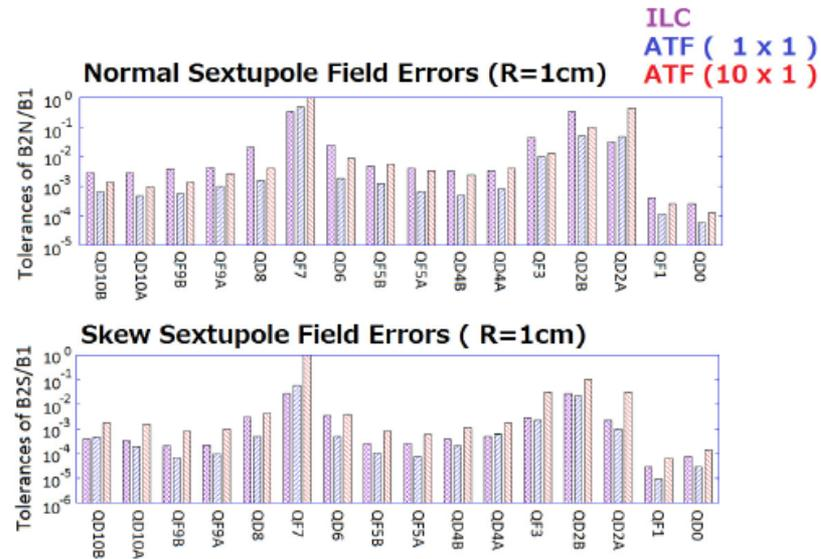
The tolerances of sextupole errors for ATF2 10x1 optics is comparable to ILC.
