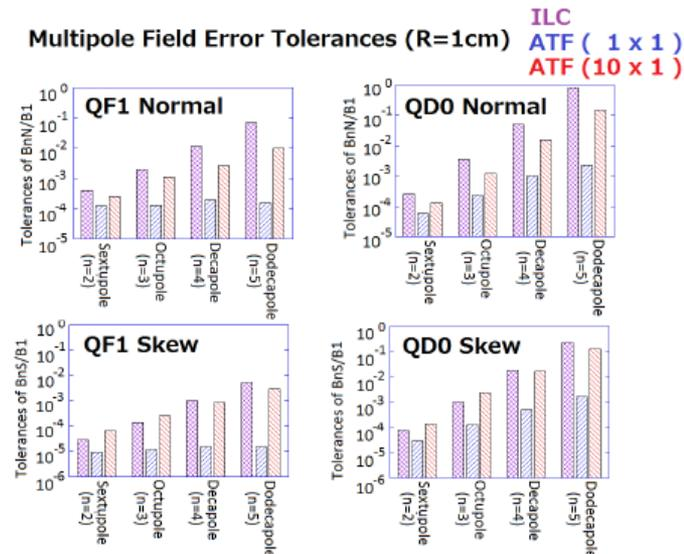
The tolerances of FD multipole errors for ATF2 10x1 optics is comparable to ILC.
