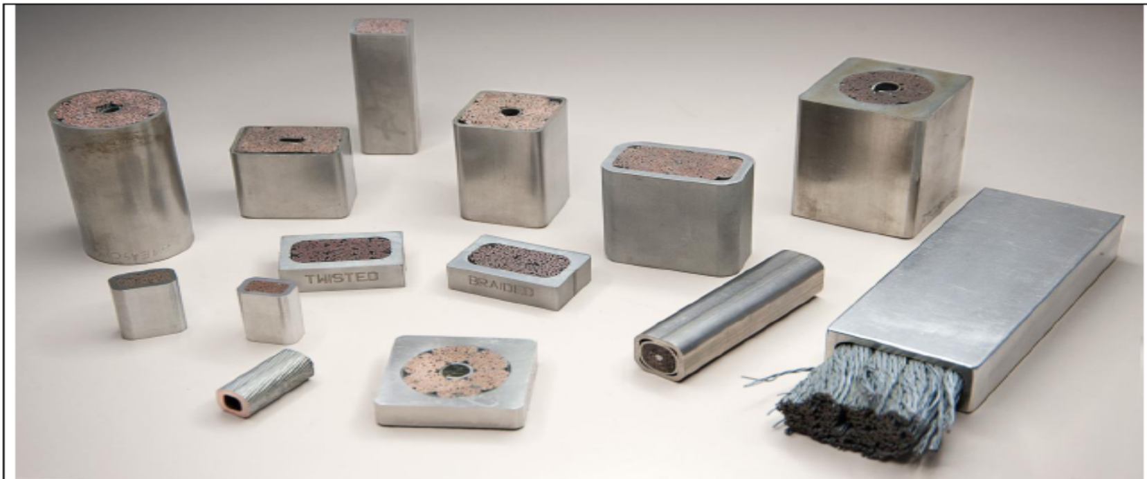
Different CICC structures manufactured for different devices
