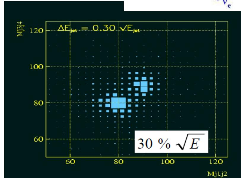
$\Delta E/E = 30\%/ \text{Sqrt}(E [\text{GeV}])$  makes W-Z separation possible
