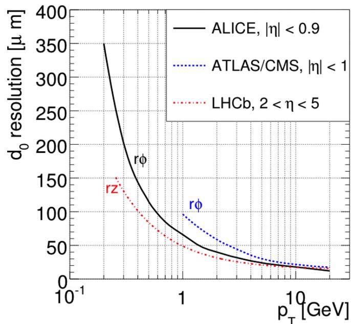
LHC detectors:  $\sigma_{r\phi} \sim 20 \mu\text{m} @ 20 \text{ GeV}$
