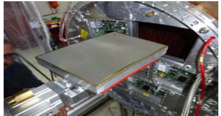
GEM and Micromegas detector as readout
