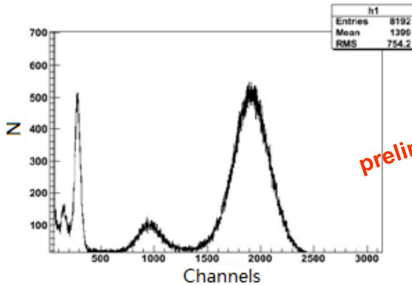
GEM+Micromegas detector's energy spectrum
