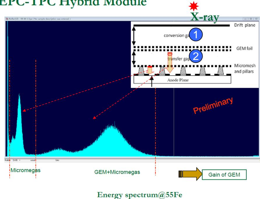
Using a CERN standard GEM and one Bulk-Micromegas assembled in IHEP
