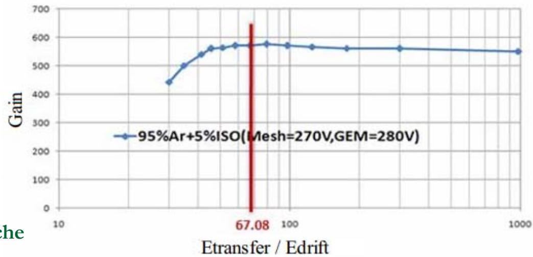
Electron transmission in GEM and Micromegas
