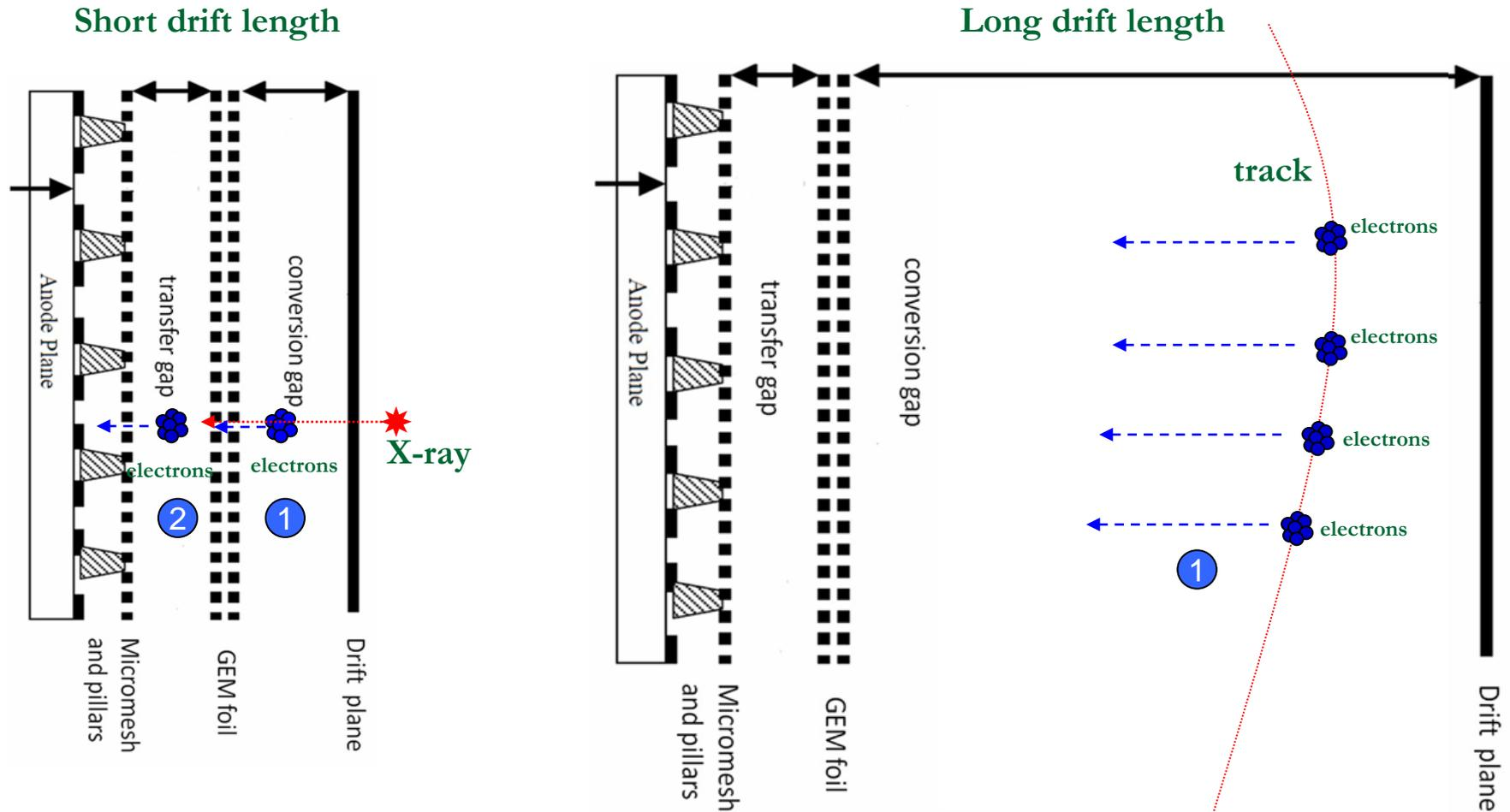
Measurement method: X-ray and particles track in the module
