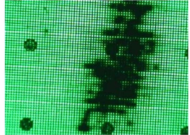
Photo of the spark damaged Micromegas
