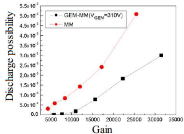
Discharge possibility VS gain @  $V_{GEM}$
