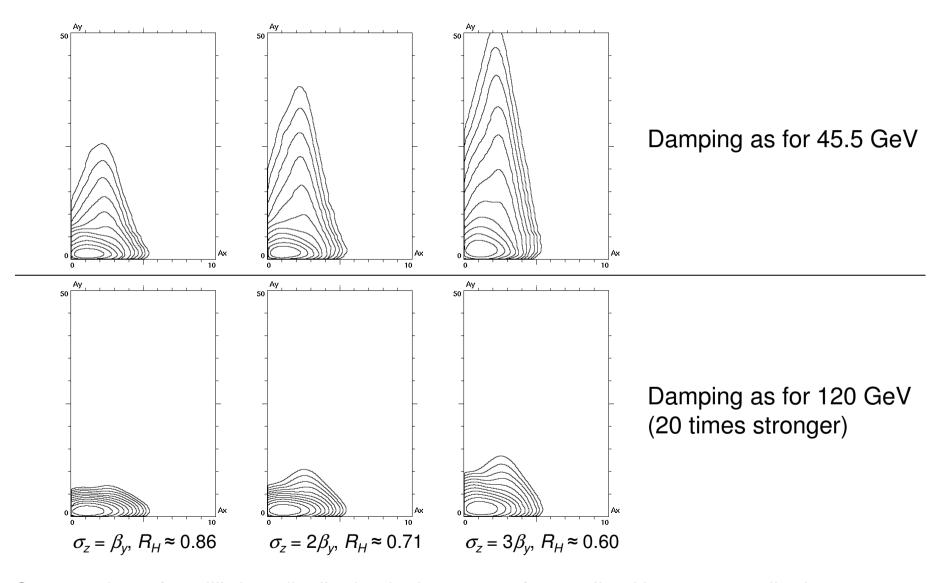
Contour plots of equilibrium distribution in the space of normalized betatron amplitudes. Density between successive contour lines decreases by a factor of *e*.
