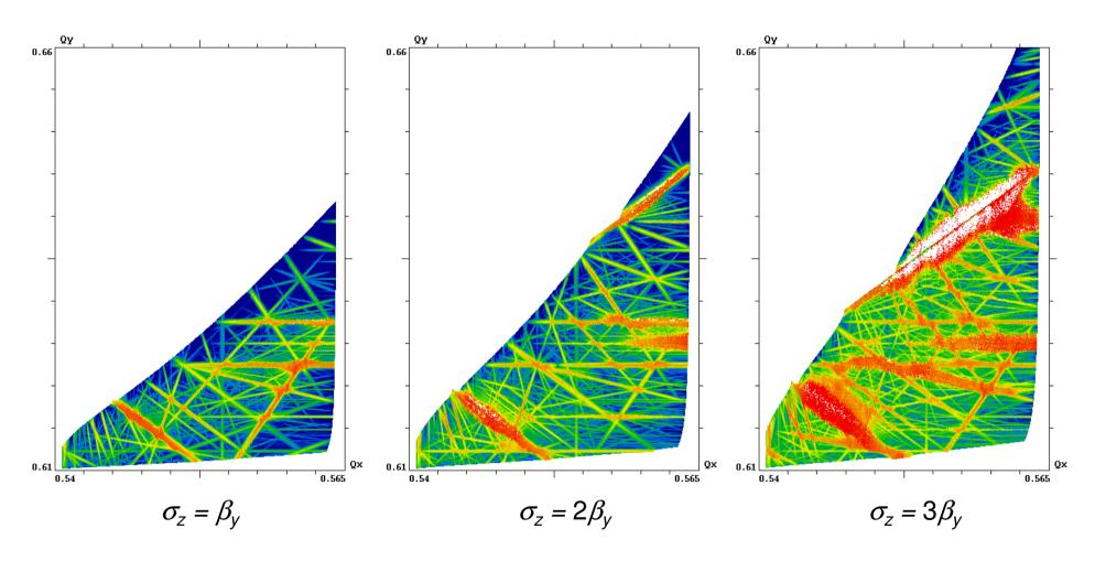
FMA footprints in the plane of betatron tunes, synchrotron amplitude:  $A_s = 1$  sigma. Parameters as for TLEP Z from FCC-ACC-SPS-0004,  $\xi_x \approx \xi_y \approx 0.03$  (nominal).
