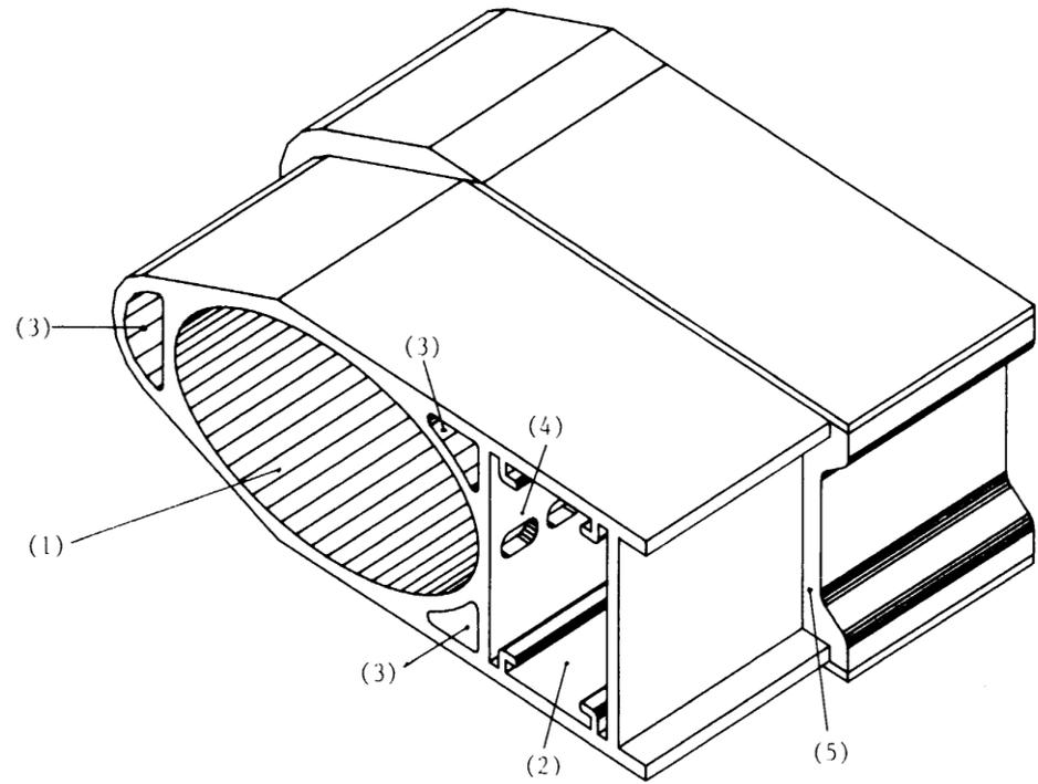
**Fig. 8.4** LEP dipole vacuum chamber, with: 1) the elliptic beam channel (131 mm × 70 mm); 2) the rectangular pumping channel where the NEG strip is mounted; 3) three cooling channels; and 4) the pumping slots. The lead shielding (5) varies between 3 and 8 mm in thickness.
