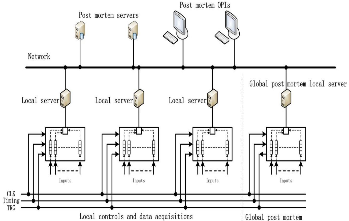
Preliminary design of post mortem recording and analysis
