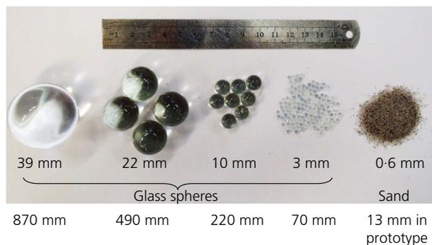
Fig. 2. Boulder and debris materials: glass spheres and Leighton Buzzard fraction C sand
