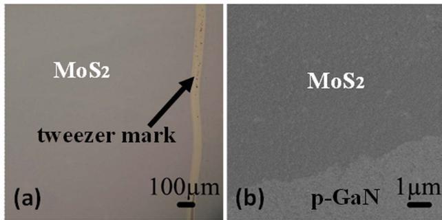
**Figure 2.** (a) Microscopic and (b) SEM images of MoS<sub>2</sub> large-area continuous multi-layer film with a scratched tweezer mark.
