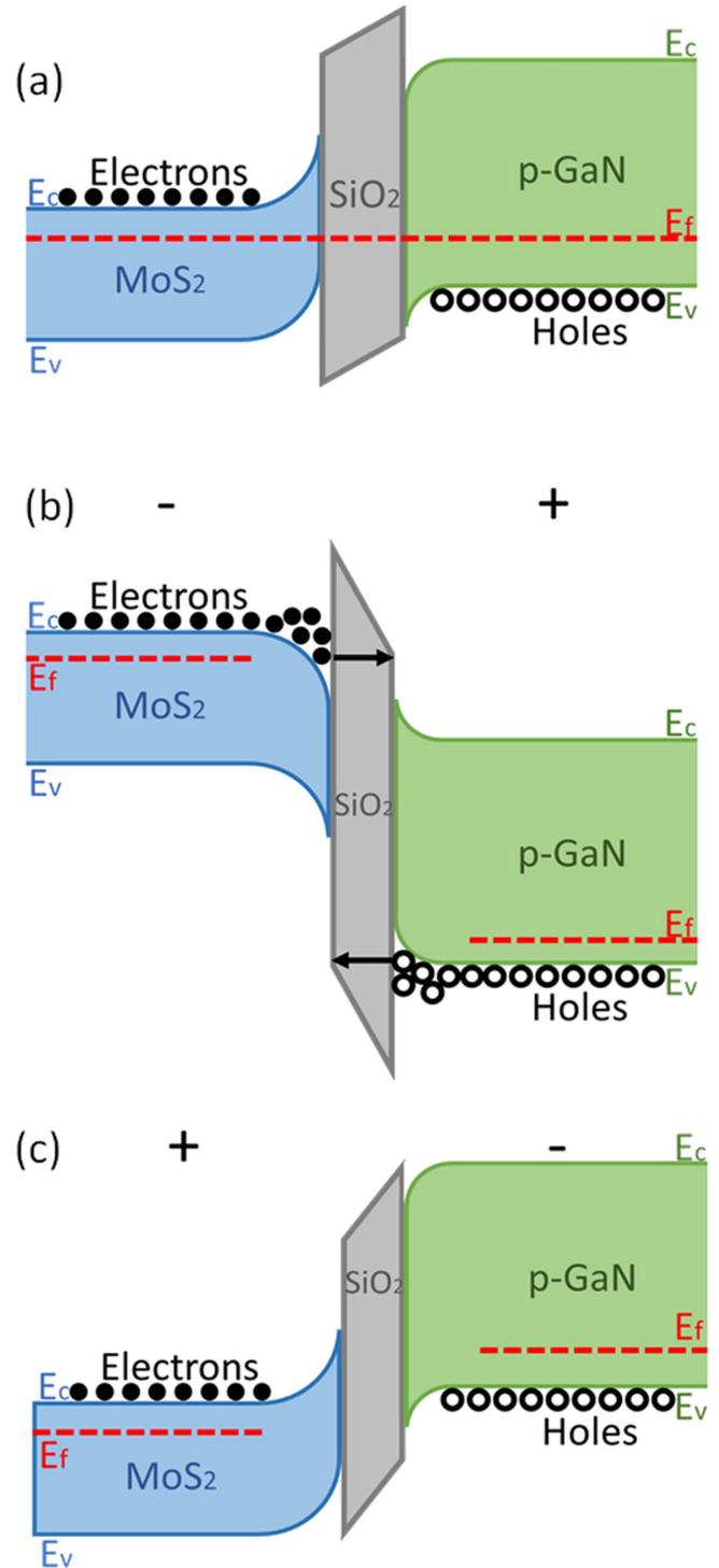
**Figure 7.** Energy band diagram of the SIS heterojunction diode at thermal equilibrium, under forward bias, and reverse bias.
