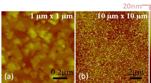
**Figure 3.** AFM images of the MoS<sub>2</sub> multi-layer film surface with scanning area (a) 1 μm × 1 μm and (b) 10 μm × 10 μm.
