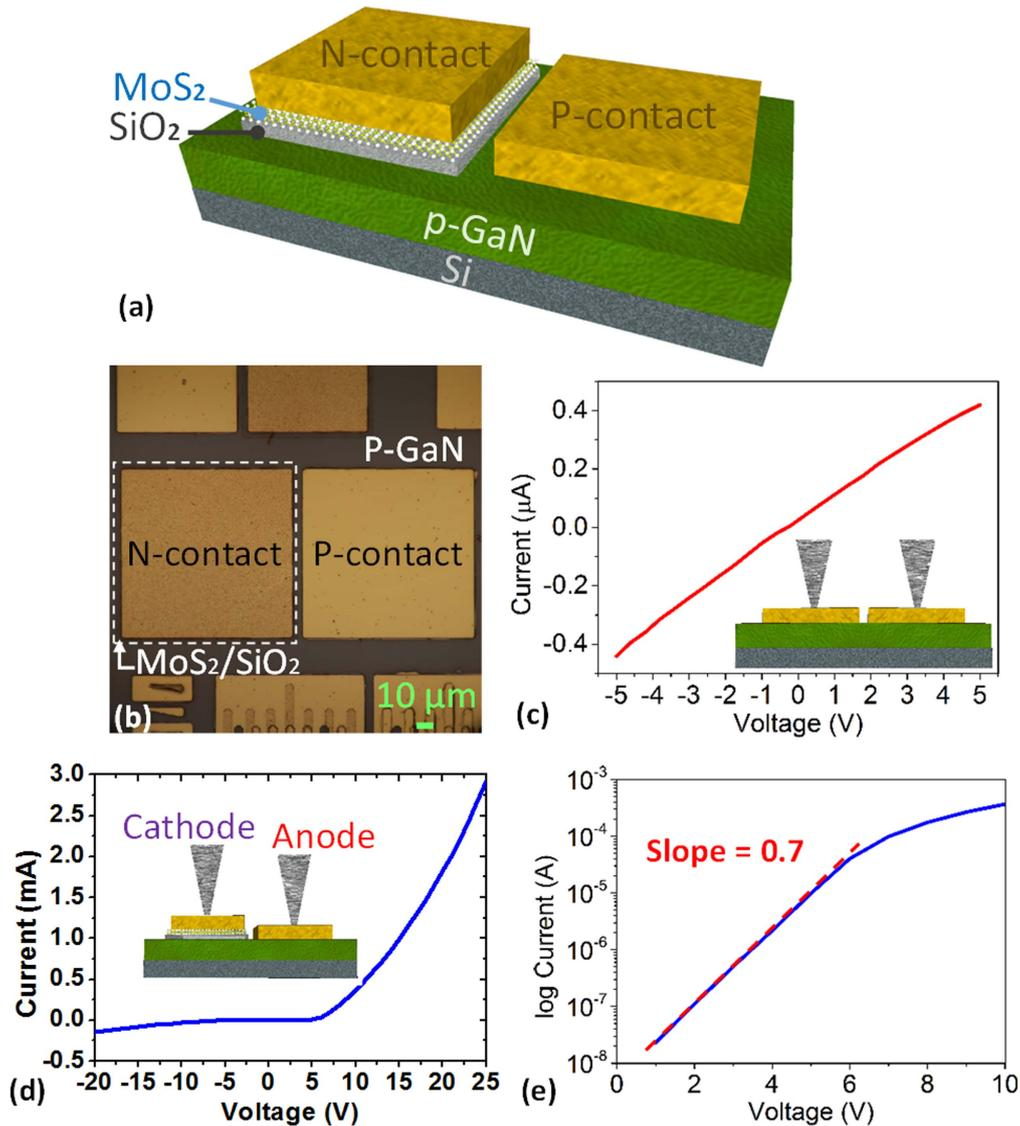
**Figure 6.** Device structure of MoS<sub>2</sub>/SiO<sub>2</sub>/p-GaN SIS heterojunction from (a) aerial view and (b) optical microscope view. Current versus bias voltage characteristics of (c) p-GaN-p-GaN contact, (d) SIS heterojunction diode in linear scale, and (e) SIS heterojunction diode in logarithmic scale.
