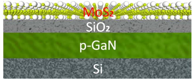
**Figure 1.** Schematic of the MoS<sub>2</sub> large-area continuous multi-layer film grown on a SiO<sub>2</sub>/p-GaN/Si substrate.
