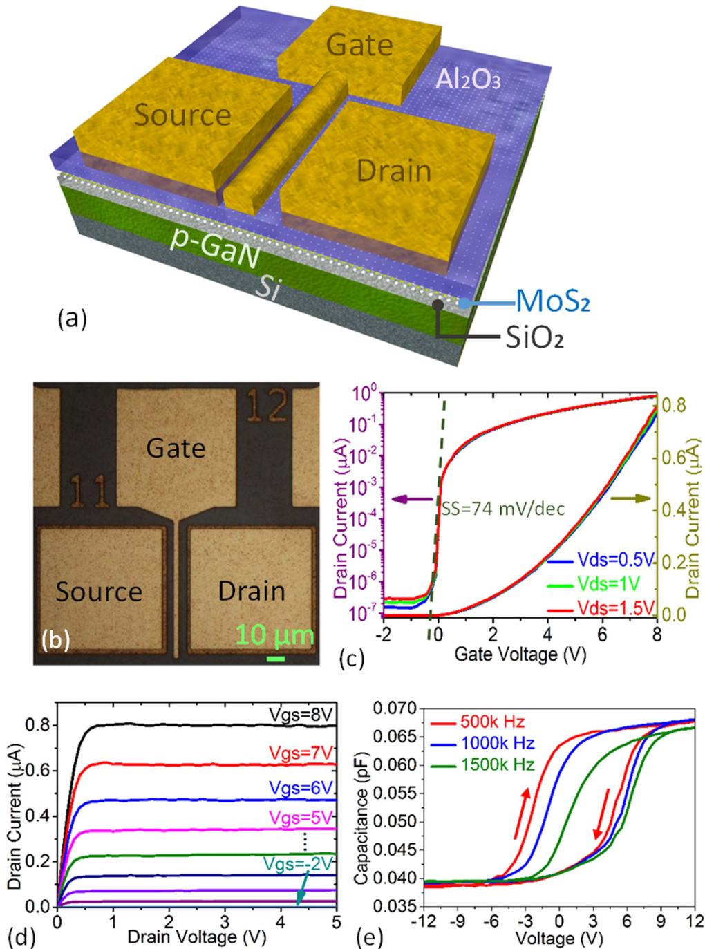
**Figure 5.** Device structure of MoS<sub>2</sub> top-gated FETs from (a) aerial view and (b) optical microscope view. (c) Logarithmic scale (left) and linear scale (right) of transfer characteristics of the MoS<sub>2</sub> few-layer film. (d) Output curve of the MoS<sub>2</sub> continuous multi-layer film FETs with several top gate voltage biases. (e) Capacitance–voltage measurement of the top-gated FETs at three different frequencies.
