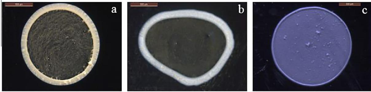
Fig. 7. Comparison of the residue patterns of 0.1 vol%  $\text{Al}_2\text{O}_3$  nanofluid of different particle sizes (a) 9 nm, (b) 13 nm and (c) 135 nm on stainless steel. The scale bar is 500  $\mu\text{m}$ .
