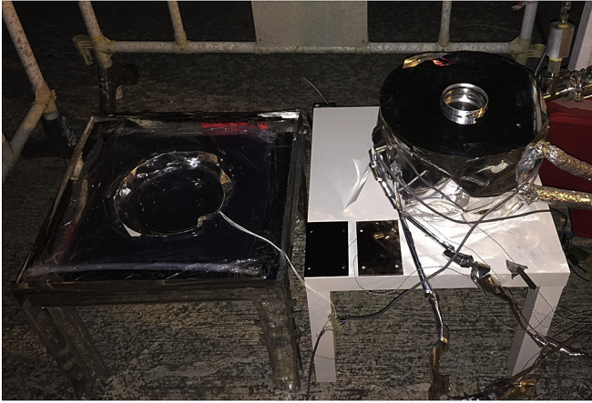
Fig. 7. Overall experimental setup of the passive radiative coolers with non-vacuum design and vacuum design with a single KCl window during night time operation.
