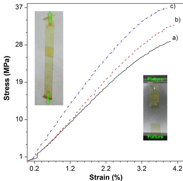
**Figure 4 | Stress-strain curves of PI films.** (a) The as-prepared film without curing, (b) the pristine film after heating at 110°C for 4 h, and (c) the self-healed film. The test was carried out at room temperature with humidity of 52% at a pulling rate of  $2 \text{ mm min}^{-1}$  by Reger-RWT10 instrument with the standard length of 20 mm. The samples were 4–5 mm in width. Inset: the healed film sample and the force direction as well as the broken site of the film after test.
