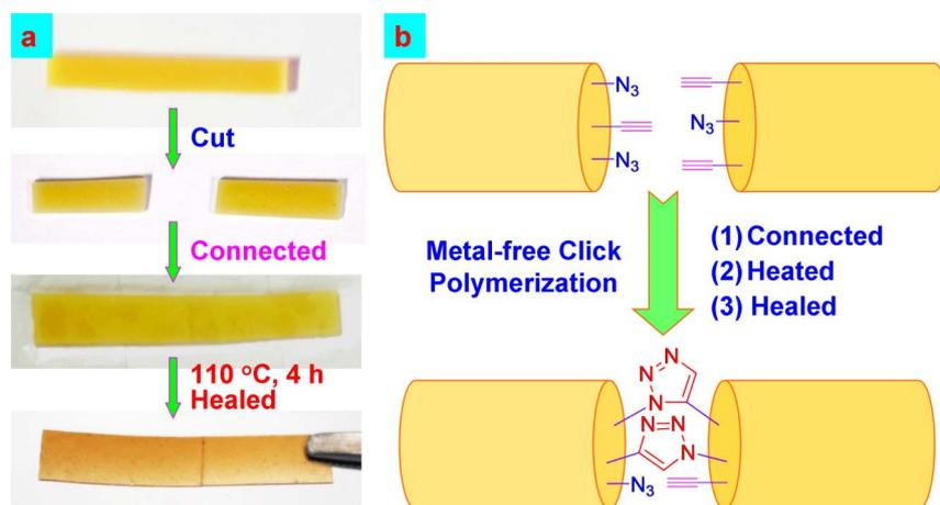
**Figure 5** | (a) The self-healing process of the PI sticks, and (b) the proposed mechanism of self-healing of polymer sticks. The sizes of the sticks are 4.10 mm in width, 1.06 mm in thickness, and 27 mm in length.
