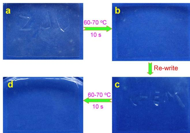
**Figure 2** | Self-repairing of the scratched surface of PI film. (a) Curved “ZJU” on the surface, (b) after heating the film, (c) re-inscribed “CHEM” on the same place of the surface, and (d) recovered surface of the film again by the same method. To better visualize the process, a blue background was used. The film is in the size of 19.9 mm × 26.3 mm.
