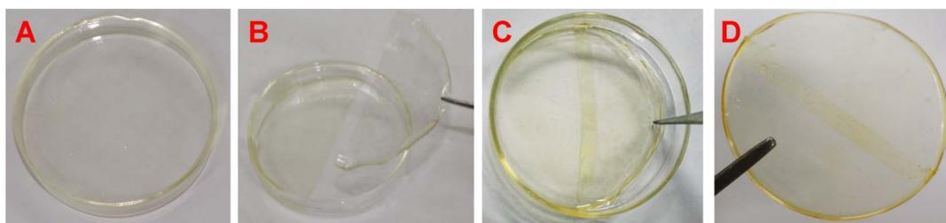
**Figure 3 | Self-healing on the surface of PI film.** (a) the as-prepared film from PI in petri-dish; (b) the half-cut film by a razor blade; (c) the self-healed film with overlapping width of 5 mm after heated at 110°C for 4 h; (d) the self-healed and stripped film. The diameter of petri-dish is 60 mm, the thickness of the as-prepared film is  $45 \pm 10 \mu\text{m}$ .
