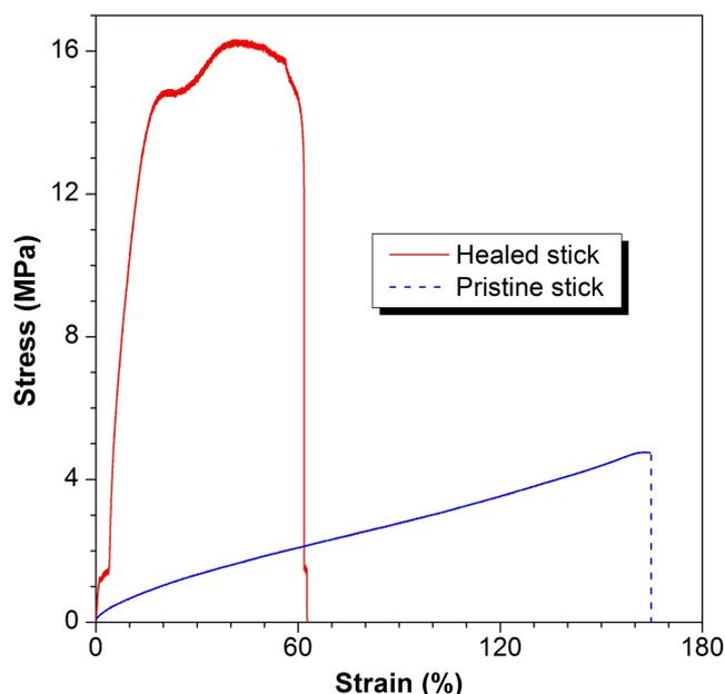
**Figure 6** | Stress-strain curves of PI sticks. (a) Before and (b) after self-healing at  $110^\circ\text{C}$  for 4 h. The test was carried out at room temperature with humidity of 52% at a pulling rate of  $2\text{ mm min}^{-1}$  by SANS CMT 4204 instrument with the standard length of 20 mm. The sizes of the sticks are 4.10 mm in width, 1.06 mm in thickness, and 27 mm in length.
