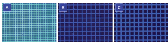
Fig. 6 Negative-tone photoresist patterns generated by photo-crosslinking of thin films of (A) P1 (sample from Table 1, no. 2), (B) P2 (Table 4, no. 2) and (C) P3 (Table 4, no. 4) through copper masks. The photographs were taken under UV illumination from a hand-held UV lamp. Square length: 100 \mu\text{m} .
