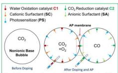
Fig 1 Concept schematic of nonionic soap bubbles doped with functional surfactants - specifically at their inner surfaces. A photosynthetic membrane will be formed at their junction generating CO & O<sub>2</sub> from CO<sub>2</sub>, water and light.
