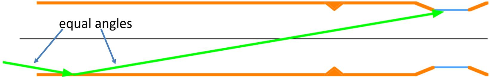
**SR photons from far upstream can possibly mirror scatter (specular reflection) off of the inside wall of the beam pipe. The angle of incidence needs to be small ( $\sim$ few mrad) and usually the photon energy is low ( $\sim$ <10 keV) but if the incident photon rate is high this can be a potential background issue. The reflection rate for this process can be >10% (see next slide)**
