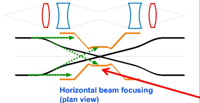
Photons generated from the final focus quadrupoles have to be masked away from the central beam pipe. The vertical focusing element is usually closest to the IP and easier to mask.
