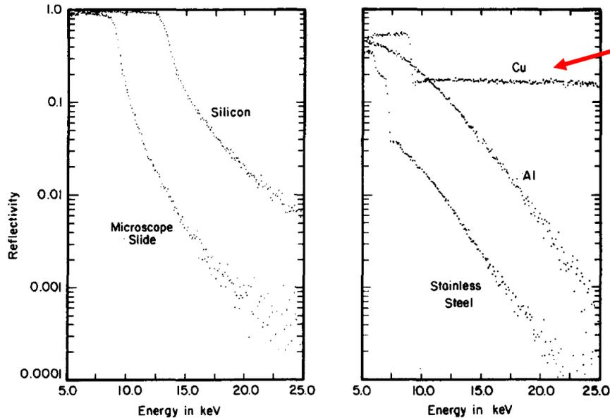
Note the high rate ( $\sim 20\%$ ) of reflectivity up to 25 keV for a 3.5 mrad incident angle on a rolled but **NOT polished** surface of Cu (typical inside wall beam pipe material)
