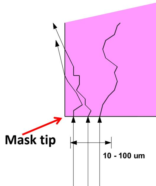
Photons that strike near the tip of a mask have a chance to scatter through the tip and then hit the central beam pipe
