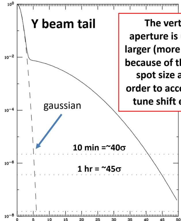
The vertical aperture is usually larger (more sigmas) because of the small spot size and in order to account for tune shift effects
