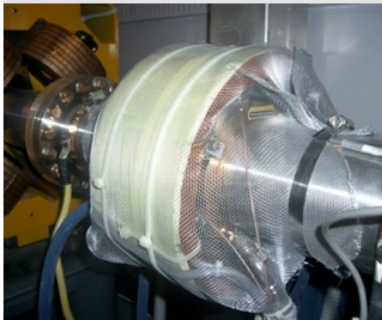
WALL CURRENT & DCCT MONITOR
