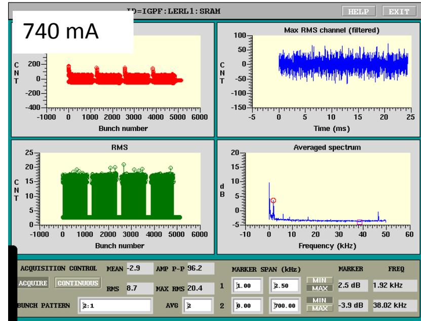
When LER beam current exceeded 830mA, a longitudinal coupled bunch instability started to be observed.
