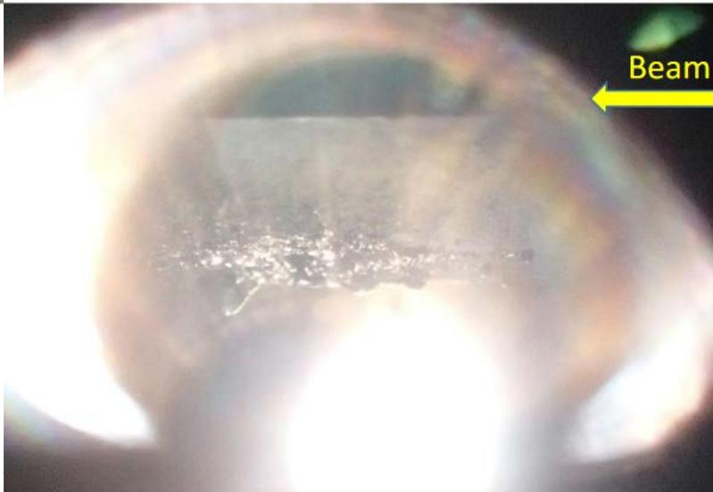
Beam hit bottom of collimator.
