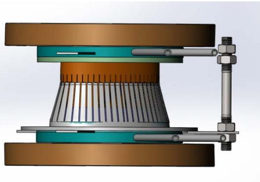
For CEPC, the fingers are designed to maintain a relatively high contact pressure of  $150 \pm 10 \text{g/finger}$ . The RF-shield should absorb the maximum expansion of 10 mm and contraction of 20 mm, allowing for the offset of 2 mm. The step at the contact point is limited to less than 1mm. The cooling water channel is attached considering the reflecting power of the synchrotron radiation, Joule loss and HOM heat load on the inner surface, and the leaked HOM power inside the bellows.
