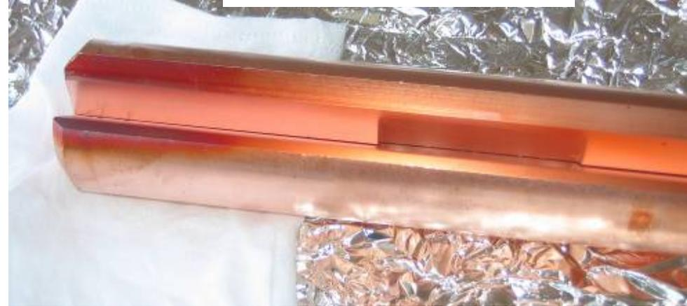
**Comparison of a leak and no-leak absorber**
