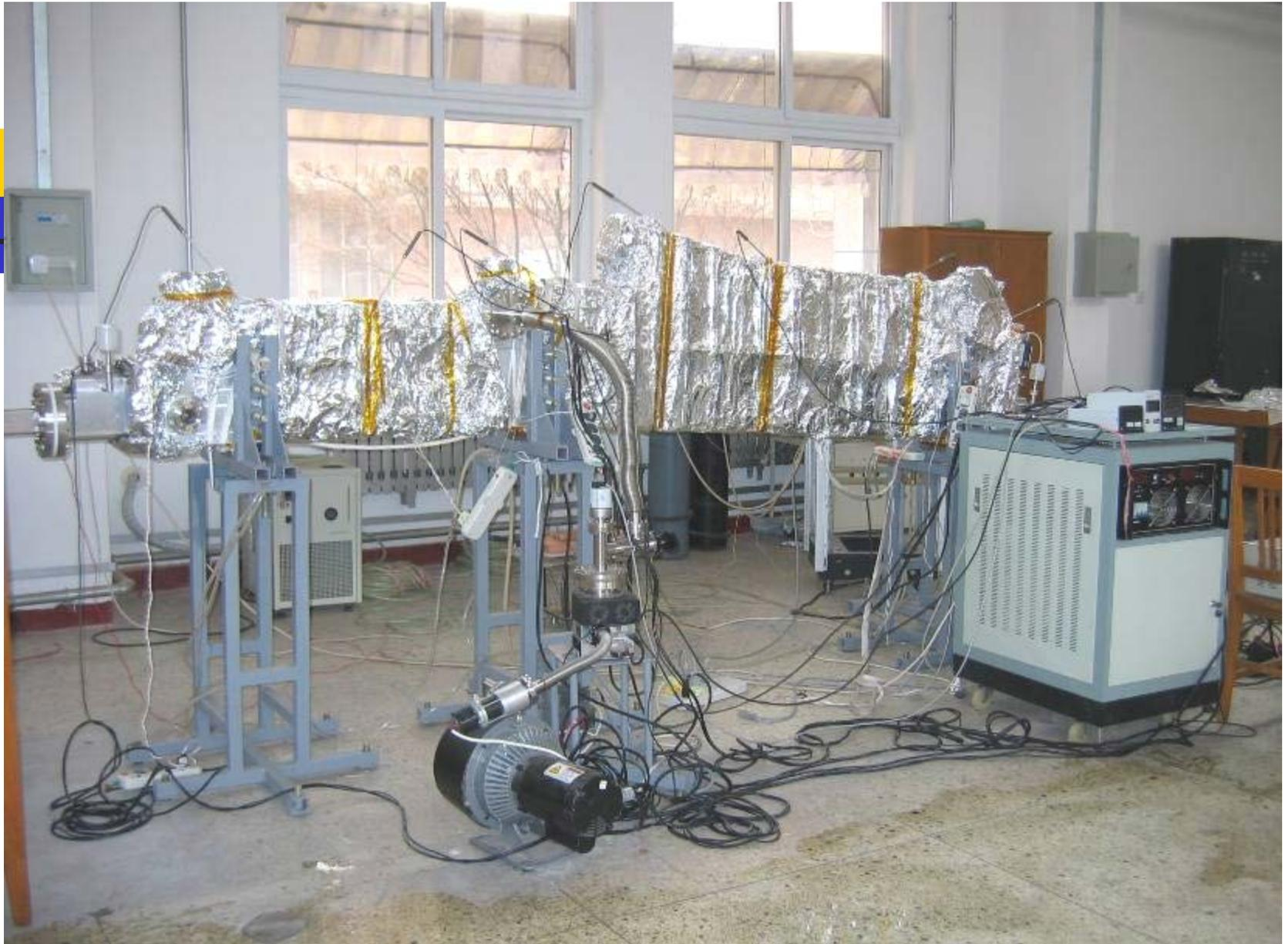
The Arc Vacuum Chamber Bakeout Before TiN Coating
