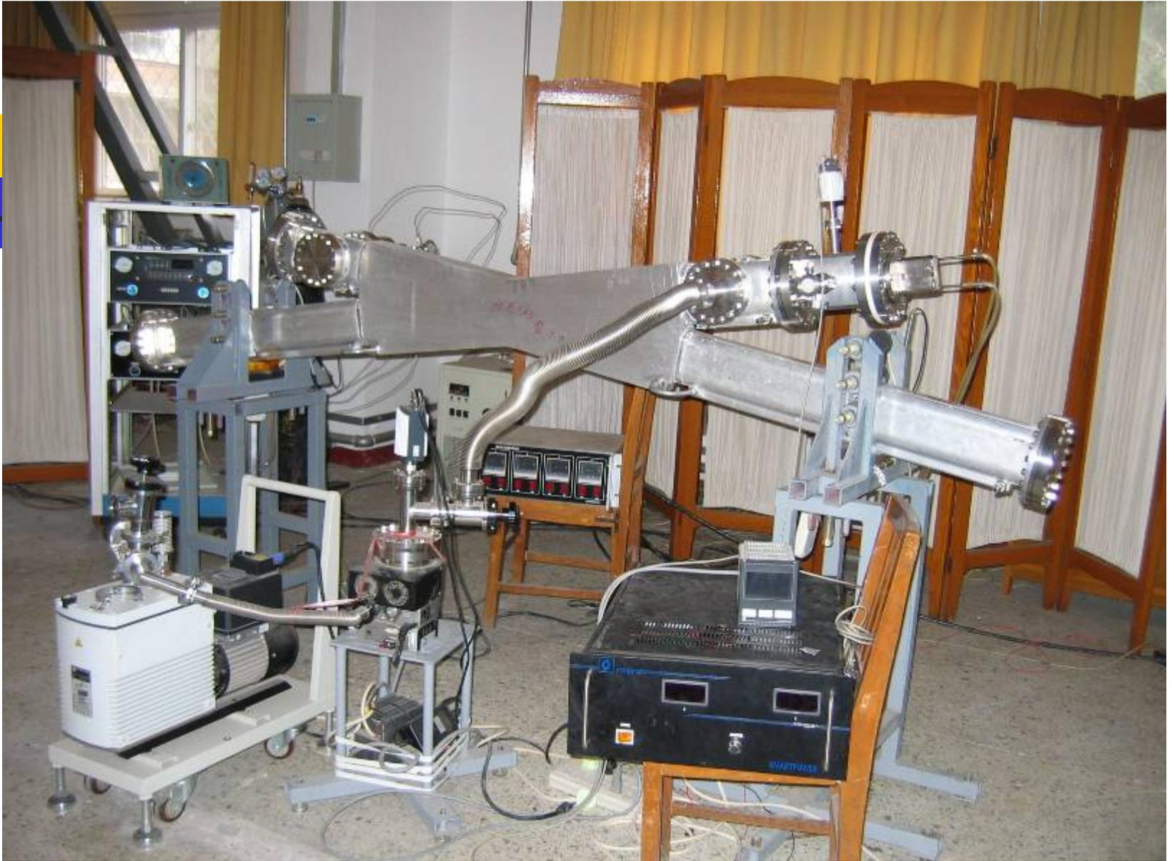
**TiN Coating Setup for the Cross Vacuum Chamber**
