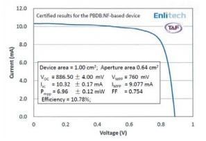
Figure 1. Photovoltaic properties of the PBDB-NF-based fullerene-free device.
