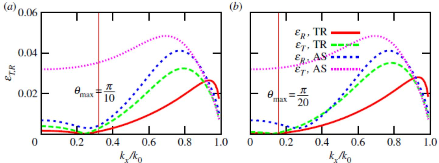
Example 1. Errors in the transmission and reflection coefficients (5.1) as functions of the sine of the incidence angle,  $\sin \theta = k_x/k_0$ , for  $a/\lambda = 0.2$ . The errors are displayed for Trefftz homogenization (TR) and for the classical asymptotic homogenization limit (AS). The maximum angles of incidence in the restricted set of basis functions for Trefftz homogenization ((a)  $\theta_{\max} = \pi/10$  and (b)  $\theta_{\max} = \pi/20$ ) are indicated by the vertical lines.
