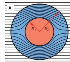
Fig. 2. A ray-tracing program has been used to calculate ray trajectories in the cloak, assuming that  $R_2 \gg \lambda$ . The rays essentially following the Poynting vector. (A) A two-dimensional (2D) cross section of rays striking our system, diverted within the annulus of cloaking material contained within  $R_1 < r < R_2$  to emerge on the far side undeviated from their original course. (B) A 3D view of the same process.
