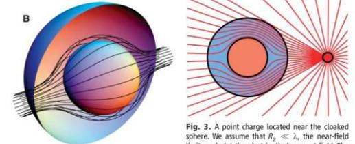
Fig. 3. A point charge located near the cloaked sphere. We assume that  $R_2 \ll \lambda$ , the near-field limit, and plot the electric displacement field. The field is excluded from the cloaked region, but emerges from the cloaking sphere undisturbed. We plot field lines closer together near the sphere to emphasize the screening effect.
