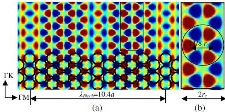
Fig. 2. (Color online) (a)  $E_z$ -field distribution of the TM-polarization Bloch wave with frequency  $0.36(c/a)$  in a 2D triangular PhC. Some air holes are denoted as black circles; (b) Field distribution of the rectangular region in (a). Each unit can be covered by a circle.
