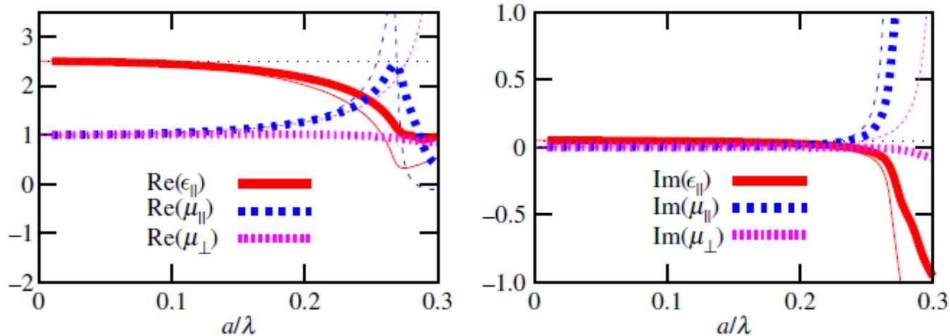
Example 1. Effective parameters by Trefftz homogenization (thick lines) and by S-parameter retrieval (thin lines) as functions of  $a/\lambda$ ; the lattice period  $a$  changes while  $\lambda$  is fixed. The dotted line represents the classical homogenization limit for  $\epsilon_{\parallel}$  (in  $s$ -polarization, the volume average of  $\epsilon_1$  and  $\epsilon_2$ ).
