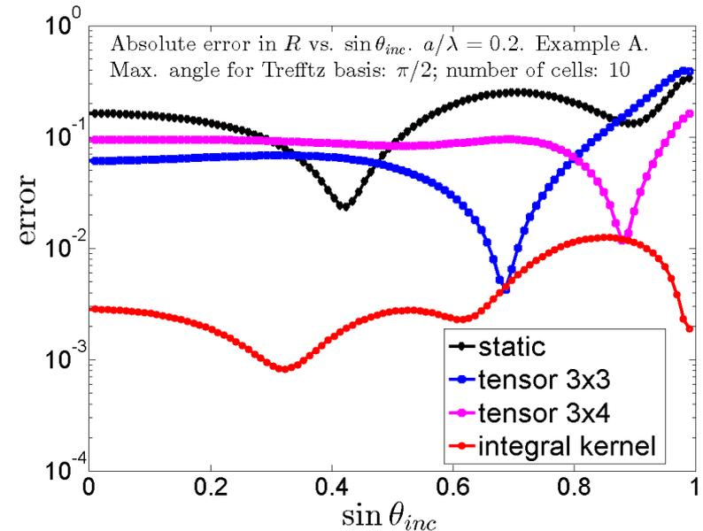
Errors in the reflection coefficient  $R$  vs.  $a/\lambda$  (left; first photonic band) and vs.  $\sin \theta$  (right). The nonlocal integral model (red line) is seen to be much more accurate than the static (asymptotic) tensor (black line) and than the local model (blue line)..
