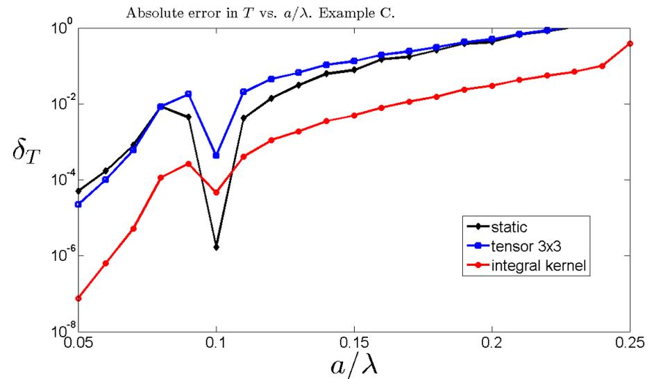
Same as before but for Example C of VM & IT, PRB 2013: Drude model for silver as material a; material b is air.  $\epsilon_0 = 5$ ,  $\omega_p = 500\gamma$ ,  $\lambda_p = 2\pi\omega_p / c \approx 136\text{nm}$ ,  $a = 0.2\lambda_p \approx 27\text{ nm}$ .
