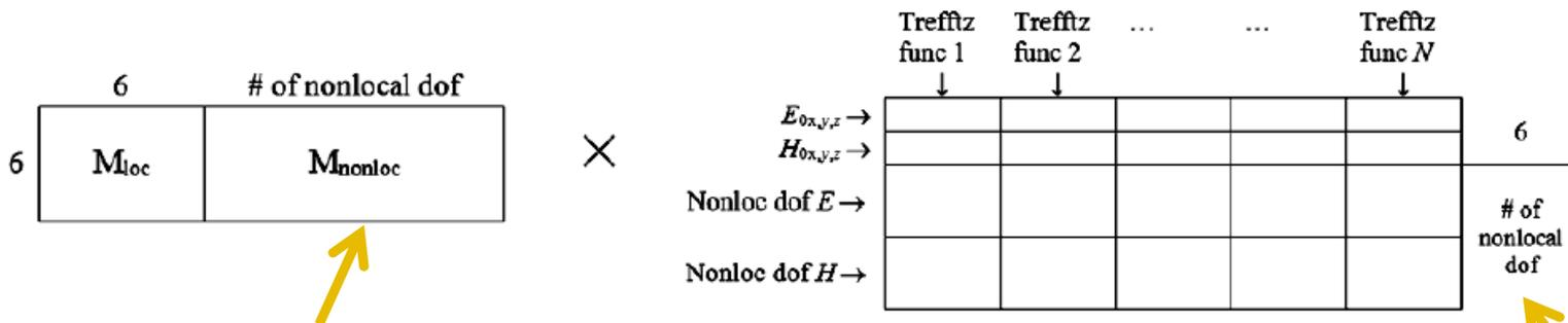
Compared to the local problem, the material tensor is expanded "rightward"
