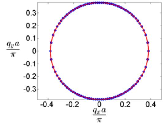
Isofrequency contour almost circular at  $a = 0.365\lambda$  (near 2<sup>nd</sup>  $\Gamma$ -point  $a \approx 0.368\lambda$ ).
