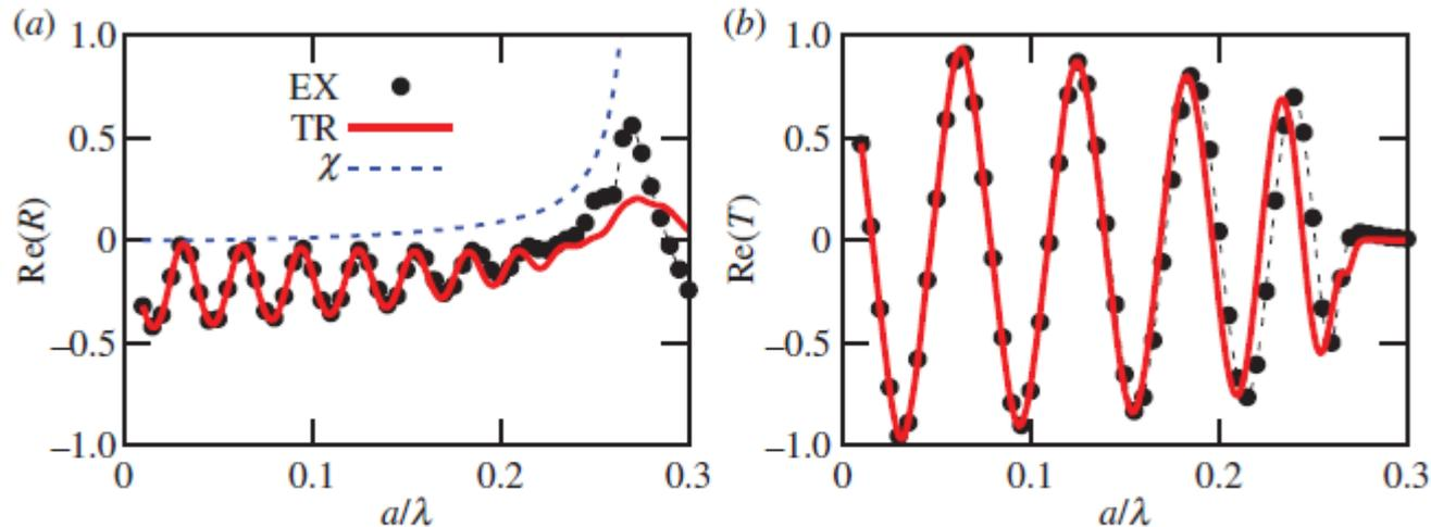
Example 1. (a) Real parts of the reflection coefficient  $R$  and (b) transmission coefficient  $T$ , and the homogenization error indicator  $\chi$  (4.2) (a) for the layered structure consisting of  $L = 10$  elementary cells and for the equivalent homogenized slab as functions of  $a/\lambda$ . EX, exact results; TR, Trefftz homogenization.
