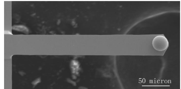
Gold coated glass sphere  $28.4 \mu\text{m}$  in diameter on the end of a cantilever
